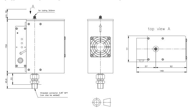
threaded bore hole, or it can be welded directly into a bore hole 17 mm ID. A PVC plug 12 mm OD is permanently linked to the mounting fitting by a thin SS stranded wire, to tightly close the fitting when the dryer has to be removed for service or repair. The maximum length of the electrical connection between the cabinet and the cooler is 10 m.
