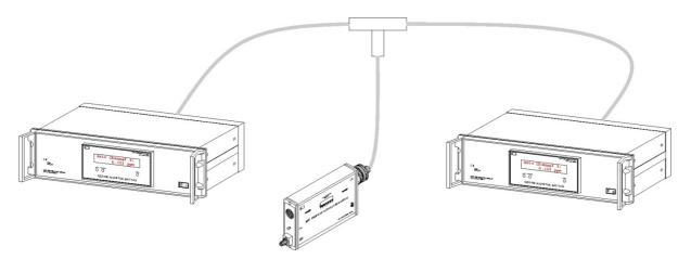
Set both monitors to a single channel in MANUAL mode. Connect two pieces of equal length to that channel of both monitors, and connect these to the TEE as shown. Use the third piece of FEP tubing to connect the TEE to the outlet of the AOS 1 through the supplied particle filter.
