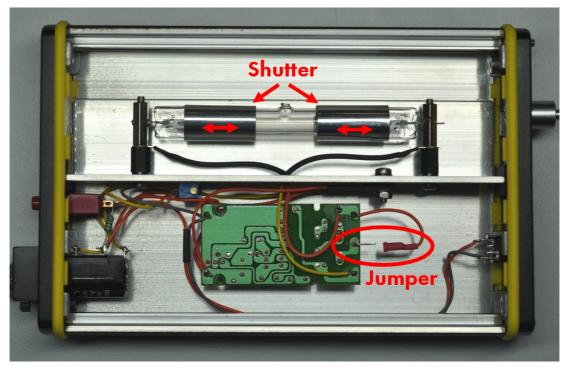
The jumper (opened in the photo) changes the electrical power passed to the UV lamp. By closing the jumper the power is doubled, compared to leaving it open.
