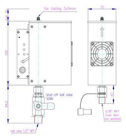
The cooler/dryer (on top of the reaction vessel) and the 24VDC/75W power supply are connected with an electric cable, and with a PTFE tubing 3x5 mm leading the sample gas from the reactor to the analyser for ozone measurement.
