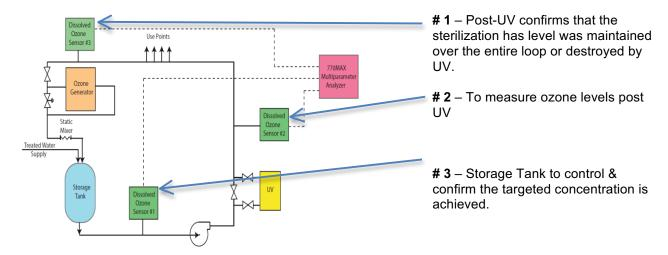
Figure 6: Dissolved Ozone Measurements (Mettler-Toledo Thomton Application Note: An-0113)
