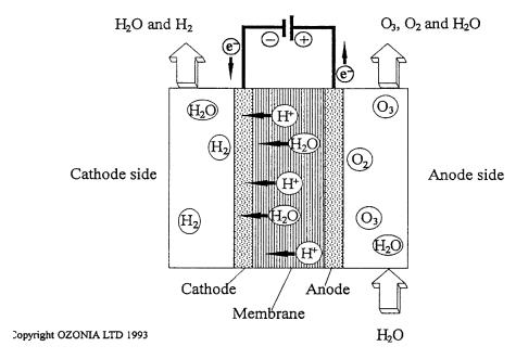
Figure 3: Electrolytic Ozone Cell
