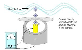
Figure 7: Polarographic Sensor
